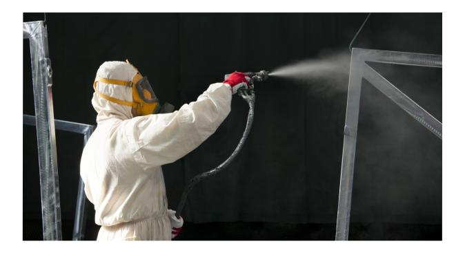
Protection with anti-corrosion coatings extends the service life of equipment and metal structures, and, as a result, cuts down costs by reducing the number of repairs and production line downtime.
